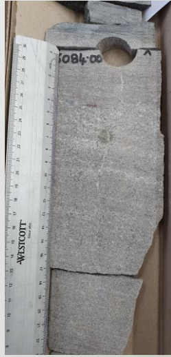
6084.5-6084.8ft Infilled fracture with bed to bed offset
