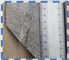
Infilled fracture clay & cement. High Angle Cross Bedding Gravel Lags.
