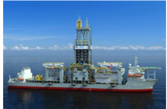
Atwood Achiever: new build 6 th generation ultradeepwater 3,650m WD drillship
